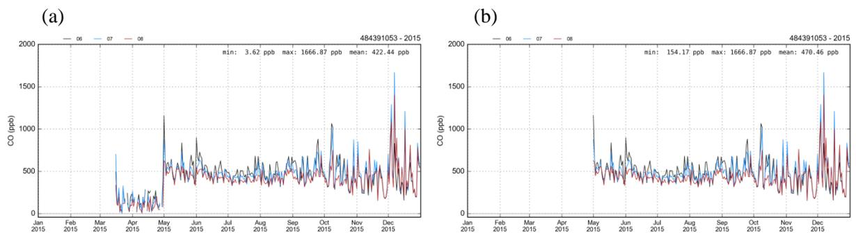
Figure 4. Preliminary time series analysis of Fort Worth near road site CO measurement data (a) with invalid data (before May 1, 2015) and (b) after the invalid data were removed.
